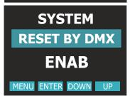
RESET BY DMX Enable: Motors reset enabled via DMX (Default) Disabled: Motors reset disabled via DMX
