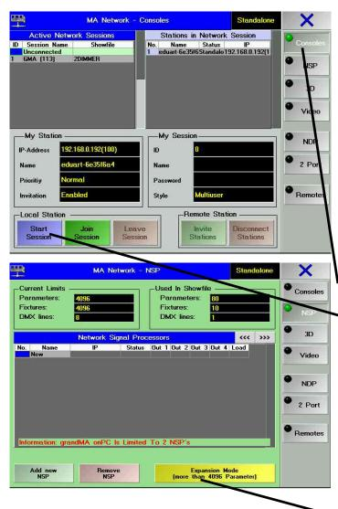
LOAD columns (numbers 0 - 100). Will show the workload of the data output of the respective NSP. If the number in this column is displayed in red, the NSP is temporarily overloaded. This will somehow decrease the normal DMX repeat rate of approx. 30 Hz. This can be disturbing e.g. with moving lamps or stroboscopes.
