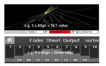
ALIGN key pressed 3 times (LED is on).
