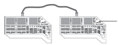
Using a "crossed" 10 Base-T cable will allow a direct console-to-console connection but no additional components can be added to this connection type later on.
