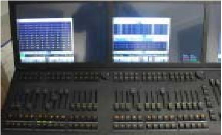
*full-size:* faders 1 - 10 are displayed on the left screen, faders 16 - 25 are displayed on th ecenter screen; faders11 - 15 and 26 - 28 are not active; faders 29 and 30 work as *Preset- and Executorfader "Set Time / Man Fade"*
