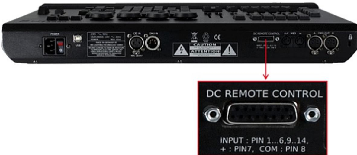
*MA onPC command wing DC remote control connector*
